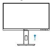
Place the monitor face down on a smooth surface. Pay attention not to scratch or damage the screen. Then lift the monitor stand.
