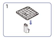
Put the stand base onto the stand neck as the direction shown in the figure.
