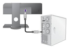
Connect the USB devices via other USB ports (downstream) on the monitor. These downstream USB ports transmit data between connected USB devices and the upstream port.
