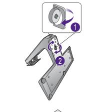
Orient and align the stand arm with the monitor, then push them together until they click and lock into place.
