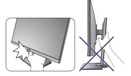
• If the monitor has been rotated to portrait mode and height adjustment is desired, you should be noted that the wide screen will keep the monitor from being lowered to its minimum height.
