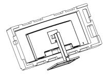
While keeping the release button pressed, tilt the base and slide it out.
