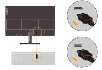
4. For computer in Analog Signal Cable connecting.
