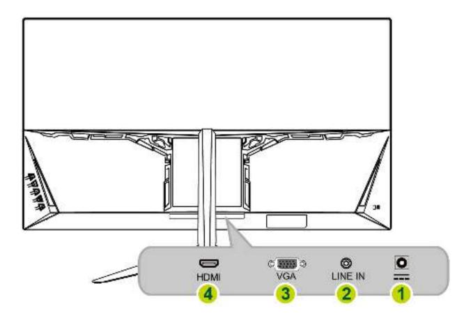
Figure.2. Connecting to a PC
