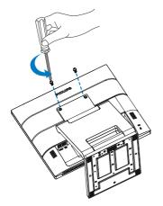
2. Move the stand into position as shown in picture. Then use a screwdriver to remove the screws, and then detach the stand from the monitor.
