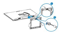
3. Remove the hinge cover from monitor body by using your fingers.
