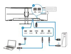
Enter to OSD menu. Go to KVM layer and select "USB up1" or "USB up2" to switch the control of peripherals from one device to another. Simply repeat this step for switching the control system using one set of peripheral.
