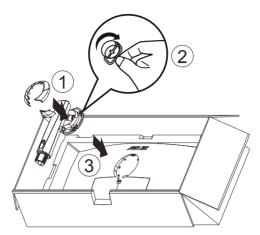
4. Fix the base to the arm by fastening the bundled screw.
