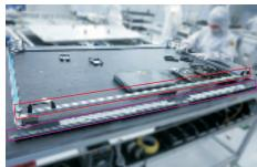
Assemble the ED holders unit with the assembled back bracket, then push the whole unit into a tripper, then fix the FFC cables with tapes, then paste 2pcs rubbers on the specific position as the picture below shown. Paste 8pcs shading tapes on the hanging ear holes of the left(4pcs) and right(4pcs) ED holder.
