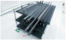
Make sure ED FFC cables are connected well, then assemble 1pcs ED holder with the assembled unit, and then use a screwdriver to tighten 24pcs(16+8) screws for locking the ED holder with the assembled unit as the picture below shown.
