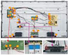
Use a screwdriver to remove 8pcs screws for S8 unlocking the two speakers. (Torque: 4.5kgf±0.5)
