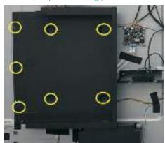
S5 Paste 1pcs for fixing the cable as the picture below shown. Remove 16pcs acetate tapes(size: 80mm) and 1pcs acetate tapes(size: 60mm) for unfixing the cables as the picture below shown.
