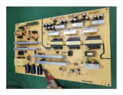
S25-4 Take out bulk cap. pin solder with soldering iron and absorber.
