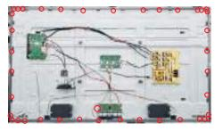
Use a screwdriver to remove 2pcs screws for S11 unlocking the key board and the holder with strip. (Torque: 2±0.3kgf)
