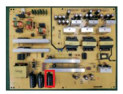
S25-1 Cut the glue between bulk cap. and PCB with a knife.
