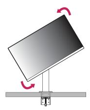
4 Complete the installation by rotating the monitor 90  $^{\circ}$  as shown in the figure.
