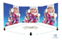
IPS displays use advanced technology that gives you extra-wide viewing angles of 178/178 degrees, making it possible to view the display from almost any angle — even in 90-degree Pivot mode! Unlike standard TN panels, IPS displays gives you remarkably crisp images with vivid colours, making it ideal not only for Photos, films and web browsing, but also for professional applications that demand colour accuracy and consistent brightness at all times.
