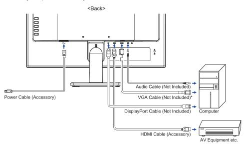
\* VGA cable is not supplied with the monitor. If you use low quality VGA cable, it may cause a result of electro-magnetic interference. Please contact the iiyama Support Centre in your country if you wish to connect the monitor via the VGA input.
