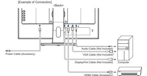
\* VGA cable is not supplied with the monitor. If you use low quality VGA cable, it may cause a result of electro-magnetic interference. Please contact the iiyama Support Centre in your country if you wish to connect the monitor via the VGA input.
