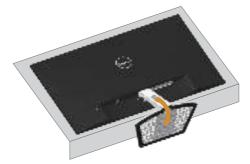
**3.** Use a long and thin screwdriver to push the release button.
