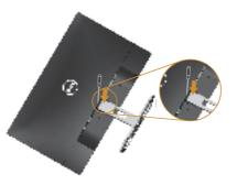
4. While pressing on the release button, pull the stand out.
