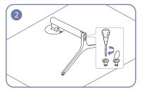
Check that the stand neck is firmly connected. Tightly fasten the connecting screw at the bottom of the stand base.
