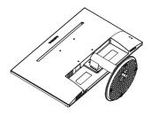
Press the release button to detach the base stand away from the base column.
