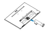
2. Hold the monitor base stand with both hands and firmly insert the base stand into the base column.
