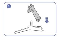
Insert the stand neck into the stand base in the direction shown in the figure.
