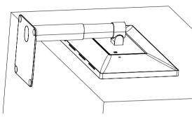
2 Push the Detach button on the back of the monitor to the left.
