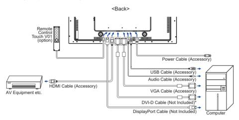
\* DVI-D cable is not supplied with the monitor. If you use low quality DVI-D cable, it may cause a result of electro-magnetic interference. Please contact the iiyama Support Centre in your country if you wish to connect the monitor via the DVI input.
