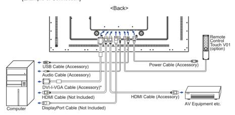
\* DVI-D cable is not supplied with the monitor. If you use low quality DVI-D cable, it may cause a result of electro-magnetic interference. Please contact the iiyama Support Centre in your country if you wish to connect the monitor via the DVI-D input.
