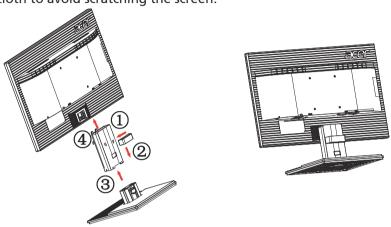
Remove: Reverse the steps to remove the base.
