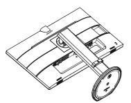
3. While keeping the release button pressed, tilt the base and slide it out.
