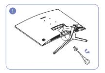
Remove the two screws to separate the stand from the screen.
