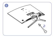
Fasten the connection part onto the screen with two screws.
