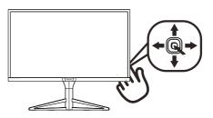
To access the OSD menu on this Philips Display simply use the single toggle button at the bottom of the Display bezel. The single button operates like a joystick. To move the cursor, simply toggle the button in four directions. Press the button to select desired option.
