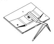
While keeping the release button pressed, tilt the base and slide it out.
