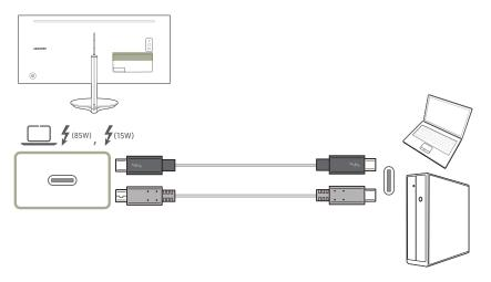
Connect the Thunderbolt™ 3 cable or USB Type-C cable to on the back of the product and on the PC.
