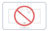
Do not hold the screen when moving or adjusting the height of the monitor. This may damage the monitor.
