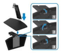
2. Align the stand-riser bracket with the grooves at the back of the monitor.
