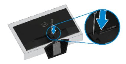
4. While keeping the release button pressed, pull the stand out.
