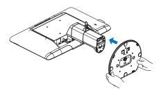
3. Attach the monitor base stand to the base column then fasten base stand.
