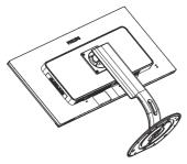
2. Loosen the assembly screws, then detach the neck from the display.
