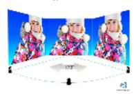
IPS displays use advanced technology that gives you extra-wide viewing angles of 178/178 degrees, making it possible to view the display from almost any angle — even in 90-degree Pivot mode! Unlike standard TN panels, IPS displays gives you remarkably crisp images with vivid colours, making it ideal not only for Photos, films and web browsing, but also for professional applications that demand colour accuracy and consistent brightness at all times.
