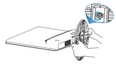
**2.** Release the screw of base stand then pull the base away from the monitor.
