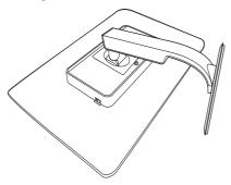
2. While keeping the release button pressed, tilt the base and slide it out.
