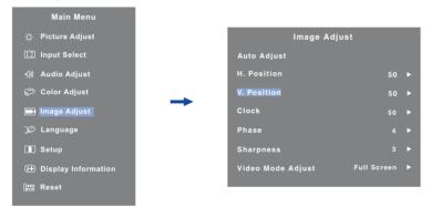
Then, use the ◀ / ▶ Buttons to change the vertical position settings. The vertical position of the overall display should be changing accordingly while you are doing this.
