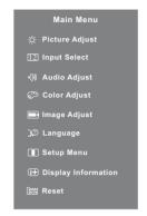
For example, to correct for vertical position, select Menu item of Image Adjust and then press the ENTER Button. Then, select V.Position by using the  $\blacktriangleleft$  /  $\blacktriangleright$  Buttons. An adjustment page appears after you press the ENTER Button.
