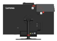
2. Screw the rear Wi-Fi antenna to the antenna connector on the rear of the computer. Then, adjust the angle of the antenna to 90 degrees.
