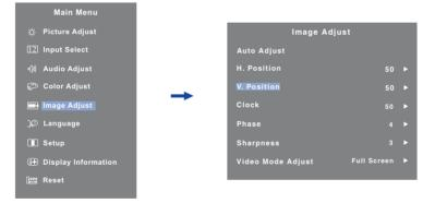
Then, use the  $\blacktriangleleft$  /  $\blacktriangleright$  Buttons to change the vertical position settings. The vertical position of the overall display should be changing accordingly while you are doing this.
