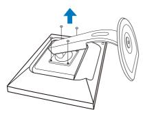
2. Remove the 4 screws and then remove the base from the LCD monitor.
