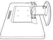
**2.** Remove the 4 screws and then remove the base from the monitor.
