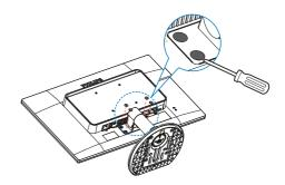
3. Remove the screws from hinge cover.
