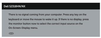
If VGA or HDMI cable is not connected, a floating dialog box as shown below appears. The monitor will enter Power Save Mode after 4 minutes if left at this state.
