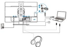
1 Kensington anti-theft lock 2 Audio input 1 Kensington anti-theft lock 3 Earphone jack 2 Audio input **4** DisplayPort input 3 Earphone jack **5** DVI input **4** DisplayPort input 6 VGA input 5 DVI input **7** AC power input 6 VGA input 8 Power Switch 7 AC power input 9 USB upstream 8 Power Switch 10 USB downstream **9** USB upstream 1 USB fast charger **10** USB downstream
