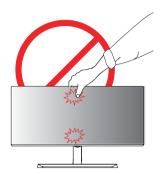
If you use the monitor panel without the stand base, its joystick button may cause the monitor to become unstable and fall, resulting in damage to the monitor or human injury. In addition, this may cause the joystick button to malfunction.
