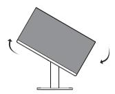
4 Complete the installation by rotating the monitor 90° as shown below.
