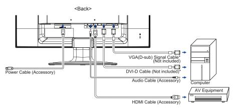
\* Cable is not supplied with the monitor; you need to use a special cable dedicated for this model. Please contact the iiyama Support Centre in your country if you wish to connect the monitor via the VGA or DVI input.
