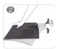
Hold the main body of the product with your hand as shown by the figure. Pull the stand in the direction of the arrow as shown in the figure to separate it.
