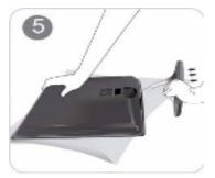
Push the assembled stand into the main body in the direction of the arrow as shown in the figure.
