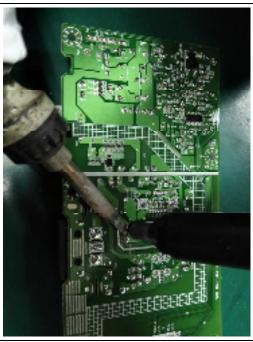
Take out bulk cap. pin solder with soldering iron and absorber
