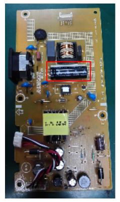
Remove electrolyte capacitors (red mark) from printed circuit boards
