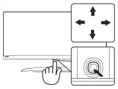
To access the OSD menu on this Philips Display simply use the single toggle button at the bottom of the Display bezel. The single button operates like a joystick. To move the cursor, simply toggle the button in four directions. Press the button to select desired option.
