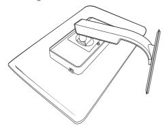
2. Remove the screws from hinge cover.
