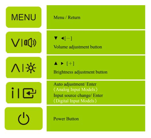
Figure.4. Control Panel Buttons
