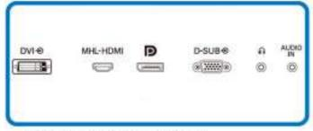
I/O back panel connector diagram
