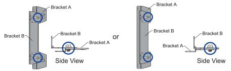
2 Depending on the monitor orientation (portrait or landscape) you choose, mount the L-Brackets to the left and right hand sides or the upper and lower sides of the monitor and tighten them with screws supplied (2 pairs of 2 pcs).
