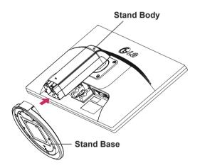
3 Using a coin, turn the screw clockwise to secure the **stand base**.
