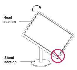
3 Be careful with the cables when rotating the screen.
